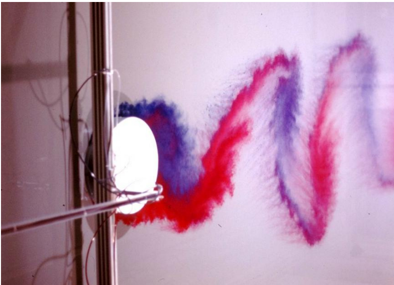
(b) Vortex street-like instability in shallow turbulent wake
